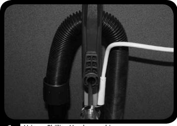
Using a Phillips Head screwdriver, remove screw from cord wrap bracket. Discard screw only.
