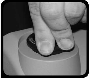
3. Quickly insert collar into bag cover evenly, pressing firmly for 20 seconds to ensure an adequate bond.
