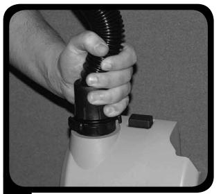
To inspect the collar, attach the quick release cuff to the bag cover collar. Lift the vacuum by the hose cuff. The collar should support the weight of the vacuum. If not, the collar will fail and separate from the bag cover. The collar will need to be removed from the quick release cuff and re-glued into the bag cover. If this collar test fails, Proceed to Step 2.
